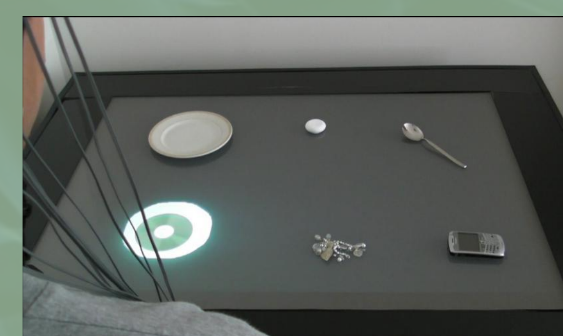
Figure 3: A participant interacting with the multi-touch table P300-based BCI. Six objects have been placed on the table. Top: The spoon is flashed by surrounding it with light. Centre: A non-object flash. Bottom: The area around the CD is being flashed.
